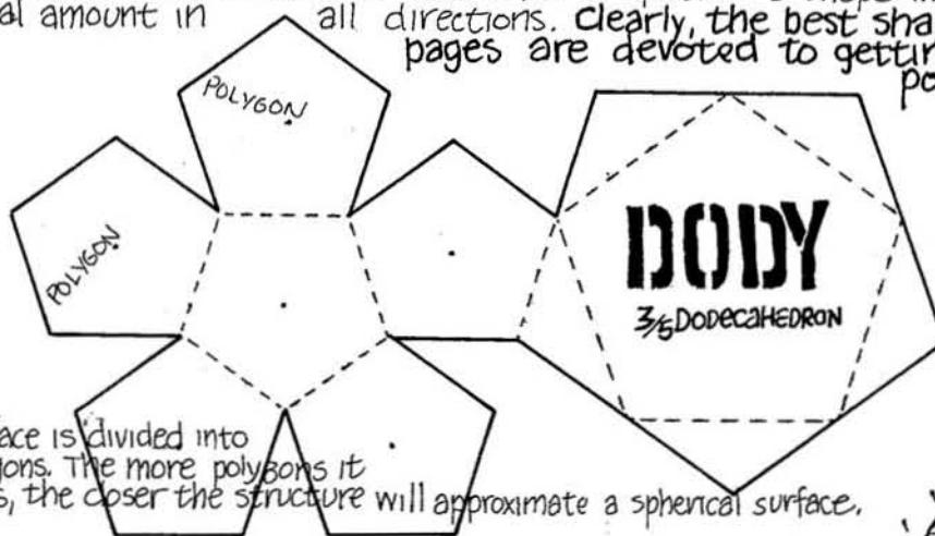
Surface is divided into polygons. The more polygons it takes, the closer the structure will approximate a spherical surface.
