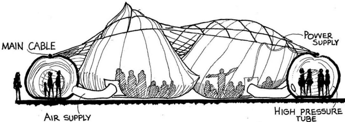
Instant Site capability, the whole packing down into four trucks. The tube provides air and access; the net when spread & tightened serves to windproof many lightweight inflatables, being built and changed according to the activities within. The main cable also provides electricity.
