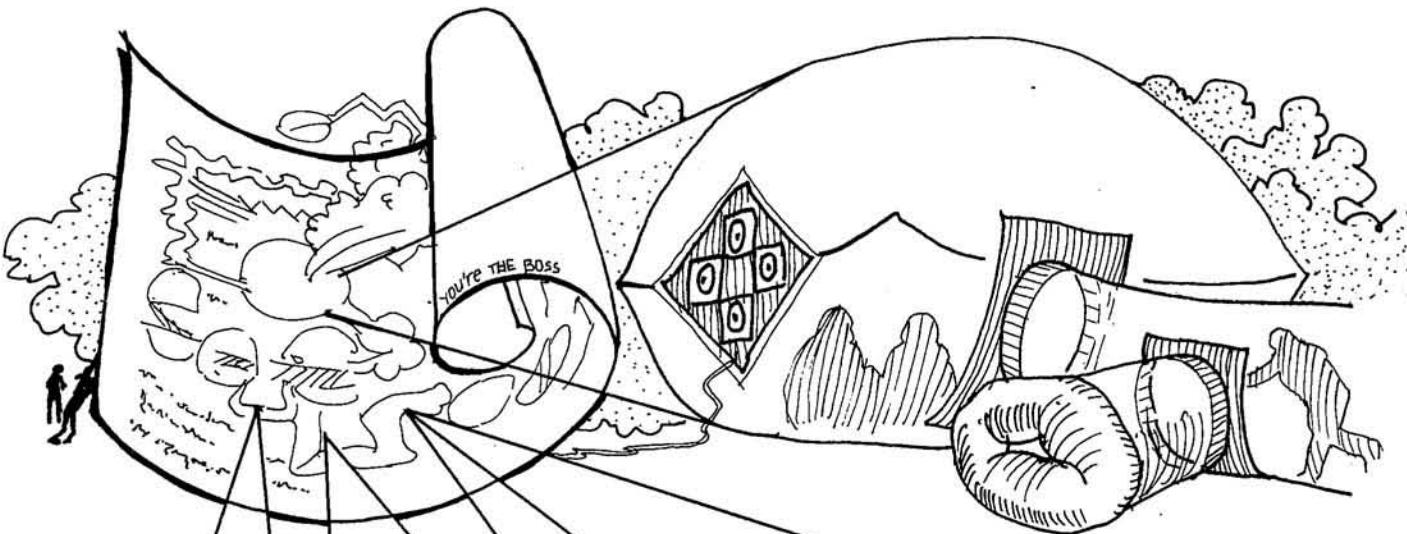
With these new Ant Farm Components you now can realize your fantasies with most of the dirty work done already. Complex curves, tube joints, fan tunnels etc. can be made ahead of time, ready to be inserted into the structure at your command. All pieces are made of high-strength vinyl, completely flexible (shown here stiffened as if inflated),
